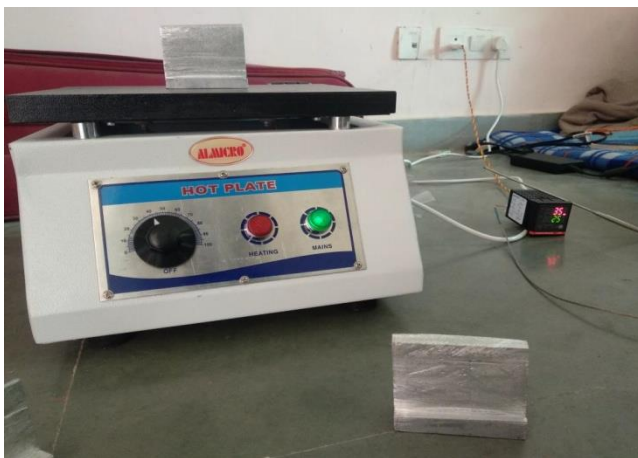
(A) Design and Fabrication of different shapes of Fins for Heat Transfer Analysis
